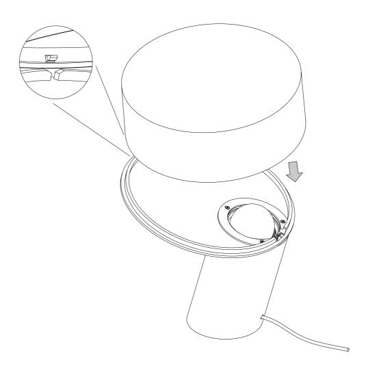
Once the shade is in place, it can be secured to the base. Insert the supplied Allen key into the two holes in the bottom and tighten the two screws that secure the shade to the base. Take care not to overtighten the screws, as this may damage some of the internal components.
