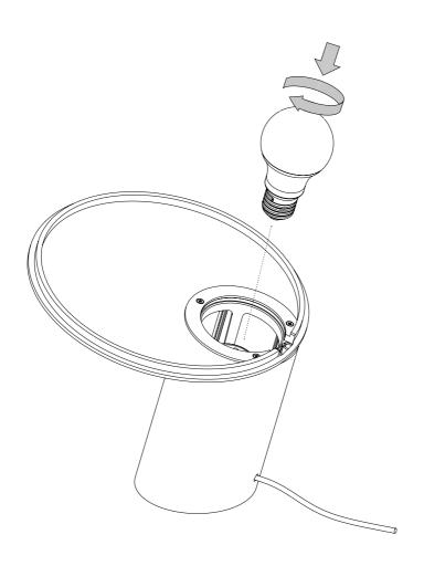
Place the shade on top of the diffuser, as shown below, aligning the small pin on the inside of the shade with the corresponding slot on the rim of the diffuser.
