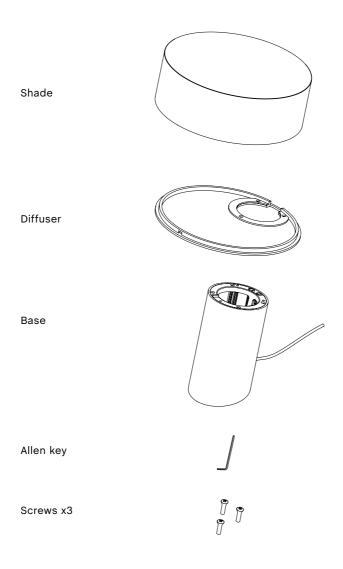
Place the diffuser on the base and insert and fasten the supplied screws, as shown below. The base has a small ridge, with a corresponding groove on the diffuser, ensuring that the two parts are correctly assembled.
